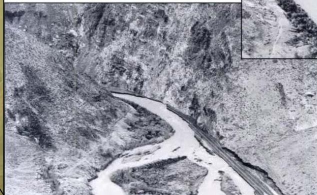
Photos 92a and 92b — Successive upstream aerial views of eastern end of Wilson Canyon, showing washed away section of S.R. 208. Photo by Nevada Department of Transportation. (Jan. 4, 1997)
